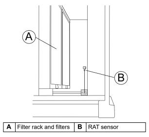
Figure 4: Factory-mounted return air temperature sensor
