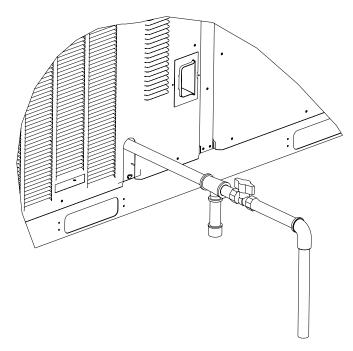
Figure 21: Side Entry Gas Piping
