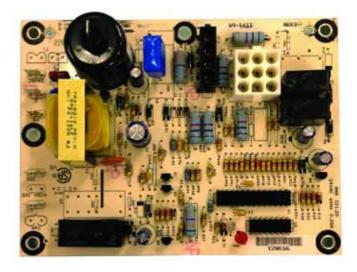
Figure 28: Ignition Control Board
