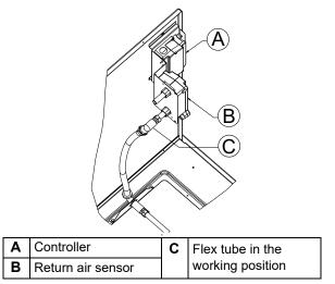
Figure 7: Return air smoke detector - working position
