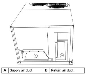
Figure 5: Supply and return air ducts
