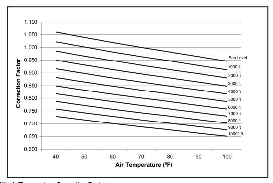
Figure 25: Altitude/Temperature Correction Factors
