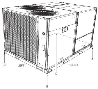
Figure 8: Unit 4 Point Load Weight
