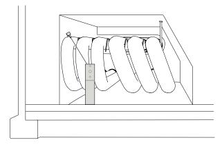
Figure 3: Supply air temperature sensor
