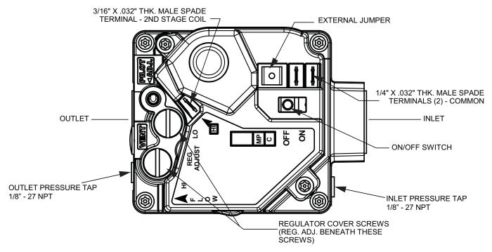
Figure 30: 6 Thru 12.5 Ton 3/4" Two Stage Gas Valve
