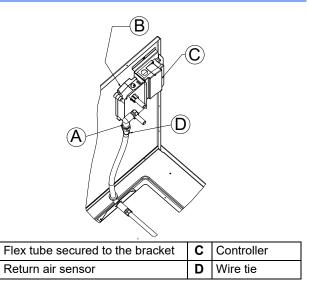
Figure 6: Return air smoke detector - shipped position
