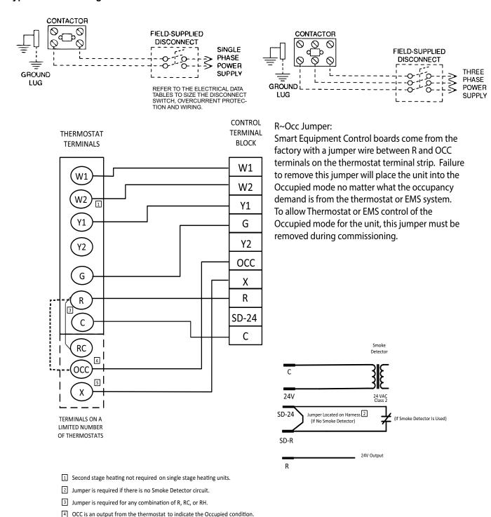
Figure 20: Typical Smart Equipment™ Control Wiring
