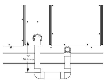
Figure 19: Condensate Drain
